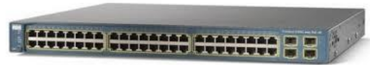
A 48 port network switch
